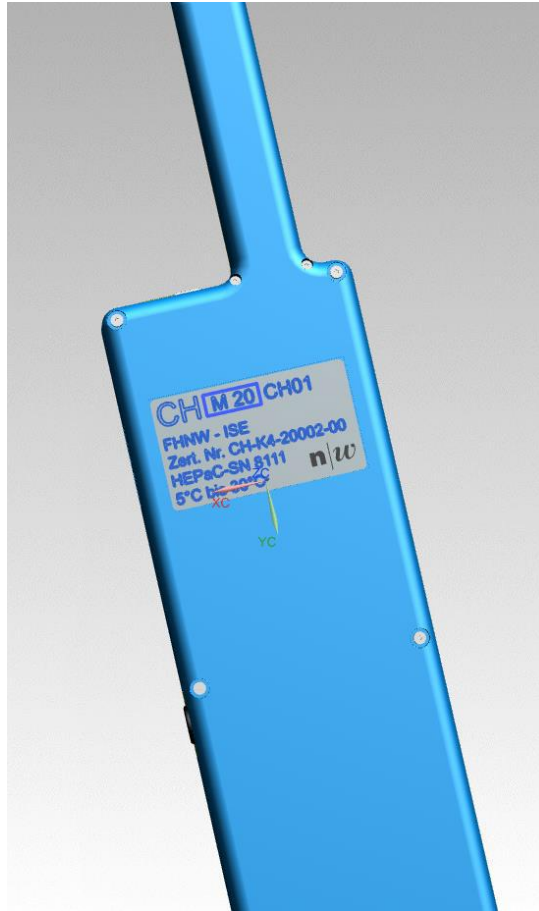
Figure 7: Position of type plate on the back of the instrument
