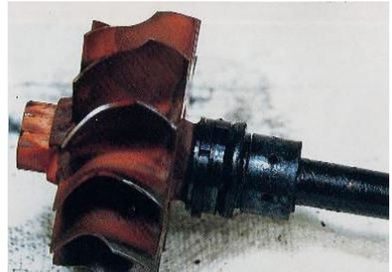
Turbine rotor with oil coking on the bearing
