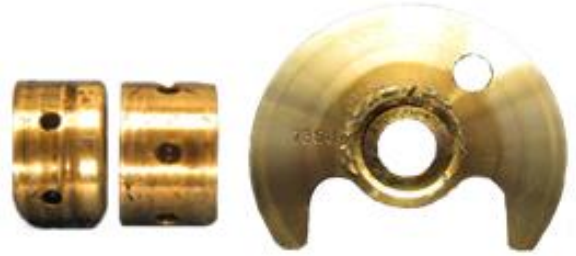
Both photos show a large amount of bearing damage due to oil starvation
